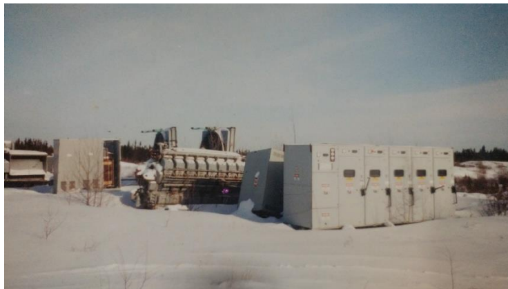
Figure 12: Generator engine, electrical panels and ventilation fans mobilized to mine site, circa 1990.
