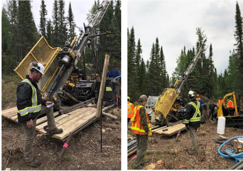
Figure 31: Diamond drill set-up of hole 18-01, twinning of hole 89-15
