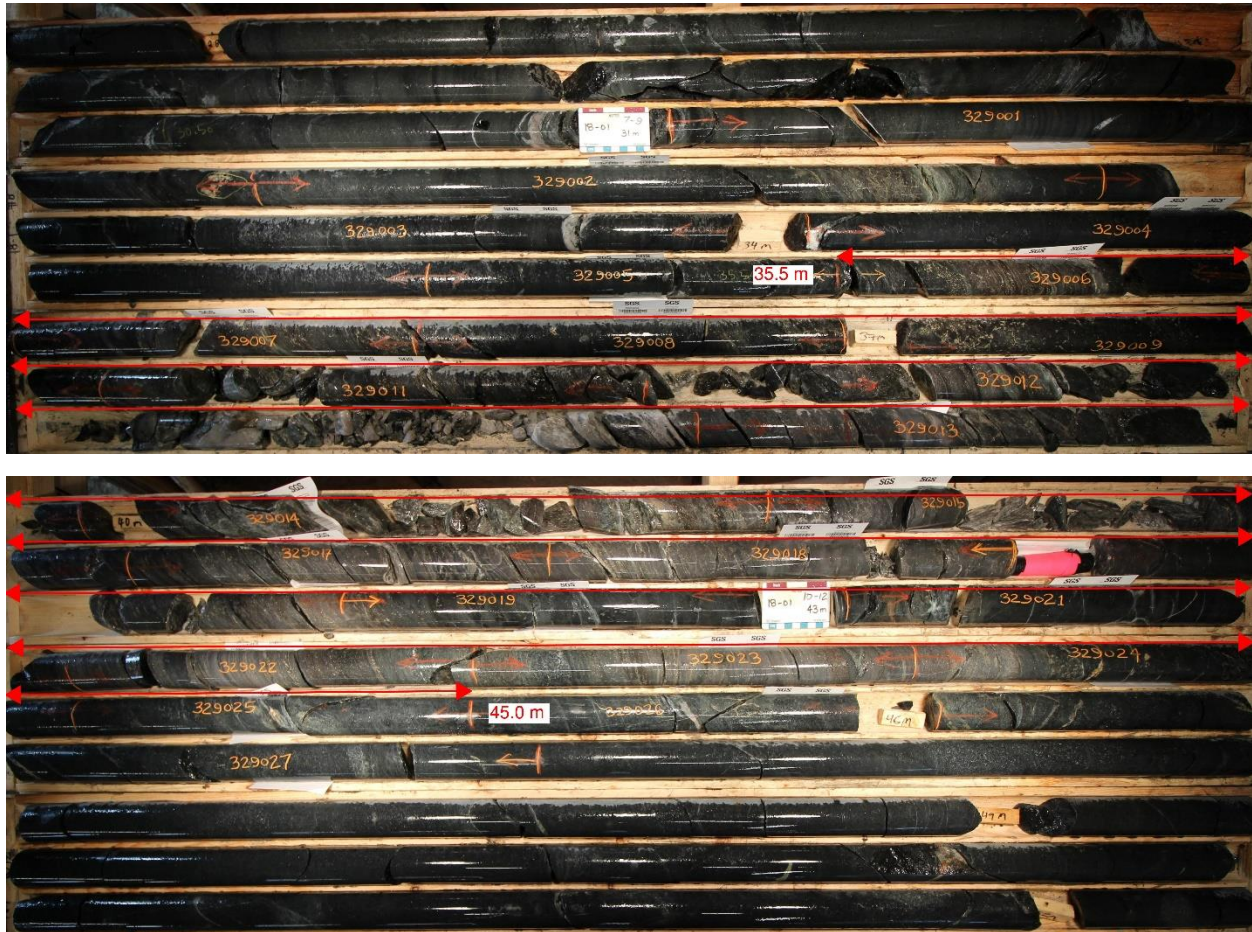
Figure 29: Drill core of West Zone mineralization. DDH 18-01 from 35.5 m to 45.0 m assayed 11.37 Au g/t (weighted average interval).
