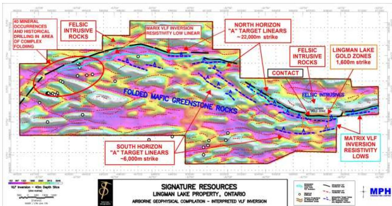
The results of the airborne survey were analyzed and shows the gold mineralized zones at Lingman Lake display correlation to both the magnetic and electromagnetic components of the survey. The Company identified an initial approximately 16 kilometers of priority target horizons for gold mineralization with 12 high priority targets that are recommended for ground evaluation along the North Horizon.
